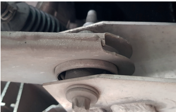
Field investigations of control arms with GEOMET® (DS3 Crossback model, year of manufacture 2019)
