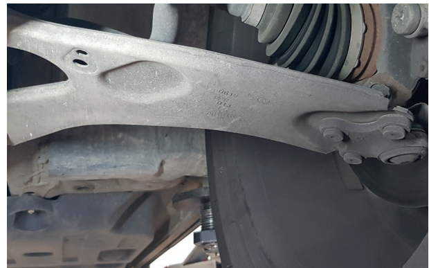
Field investigations of control arms with GEOMET® (DS3 Crossback model, year of manufacture 2019)
