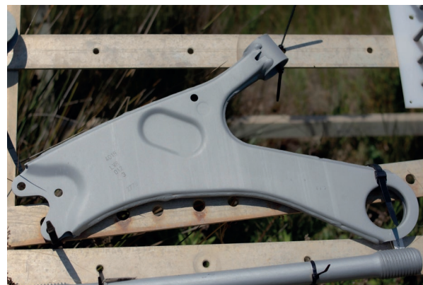
Control arm in outdoor weathering (maritime climate) after 60 months.
